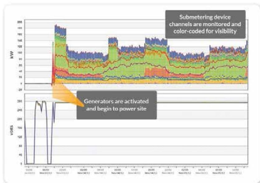
**Figure 3.** Ensure sites are receiving generator power with detailed visibility of voltage levels.
