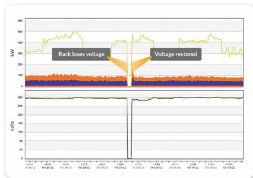
**Figure 5.** The energy manager monitors refrigeration rack voltage performance.
