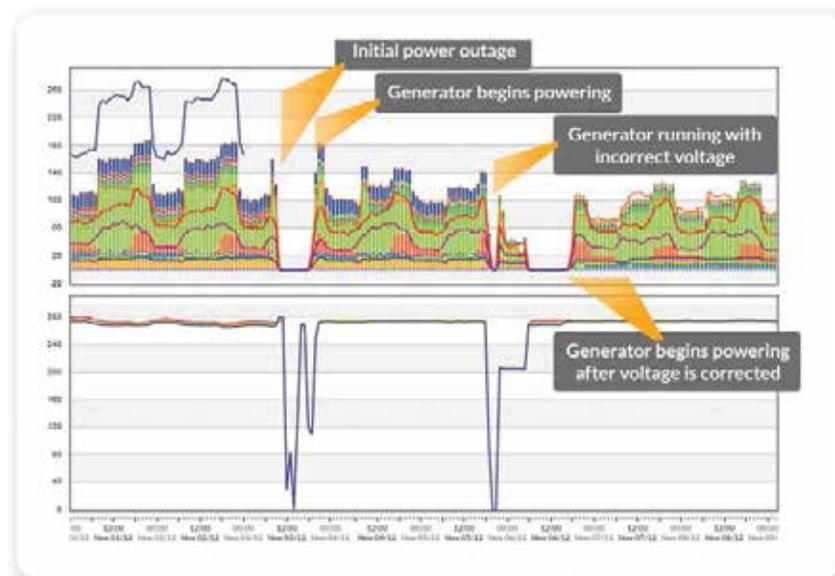
**Figure 4.** The energy manager details generator performance.
